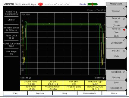
Figure 2-4. GSM Power vs. Time (Slot) Measurement
