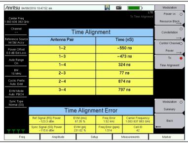
Figure 5-9. Tx Time Alignment (4x4 MIMO Configuration)
