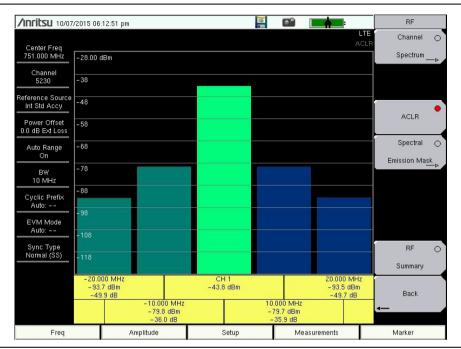
Figure 5-3. Adjacent Channel Leakage Ratio
