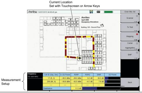
Figure 7-2. Indoor Coverage Mapping (GPS Off)
