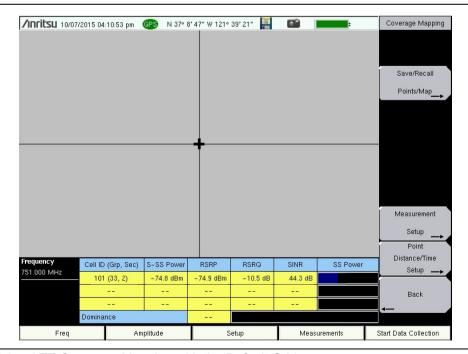
Figure 7-3. LTE Coverage Mapping with the Default Grid
