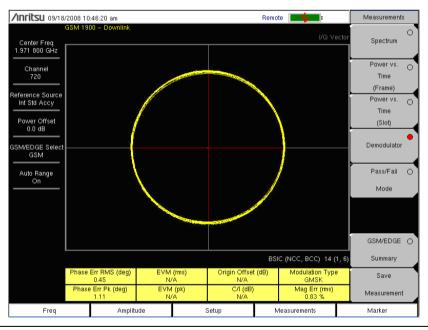
Figure 2-5. GSM Demodulator Measurement
