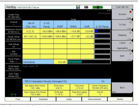
Figure 5-12. Over-the-Air Scanner Measurements
