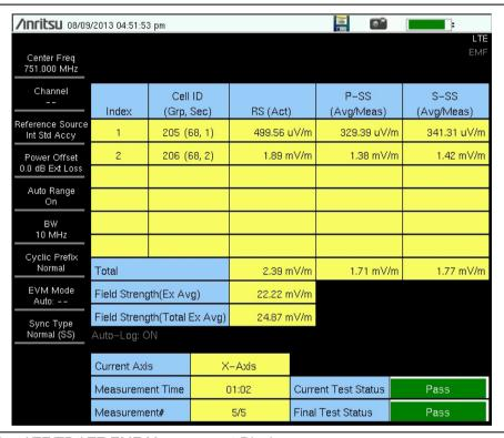
Figure 8-8. LTE/TD-LTE EMF Measurement Display
