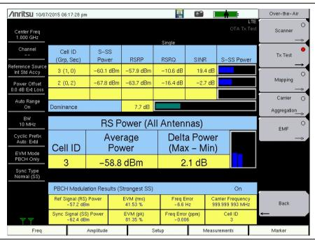
Figure 5-13. Over-the-Air Tx Test Measurement
