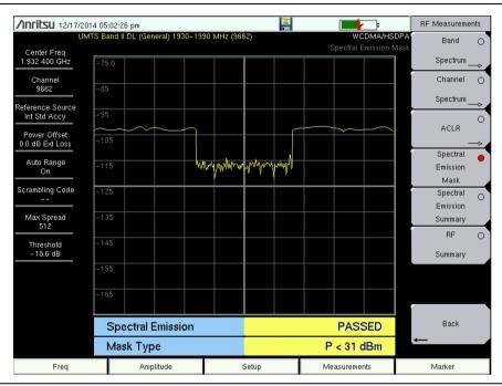
Figure 3-5. Spectral Emission Mask Measurement
