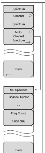
**Channel Spectrum:** Displays the spectrum of the selected channel. The screen also displays Channel Power, Occupied Bandwidth, Frequency Error in PPM and Hz, Burst and Average Burst Power, and the Base Station Identity Code (BSIC).
