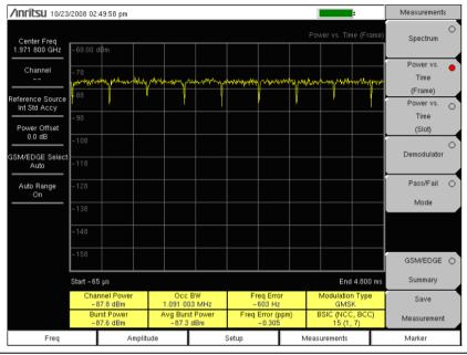
Figure 2-3. GSM Power vs. Time (Frame) Measurement
