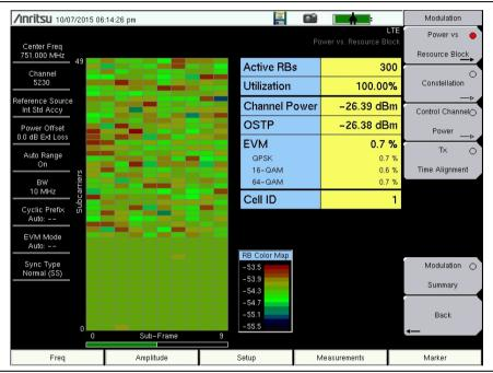
Figure 5-6. Power versus Resource Block Measurement View
