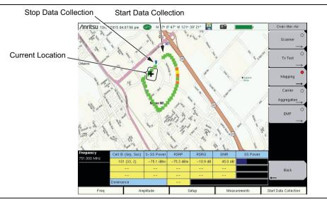
Figure 7-1. Outdoor Coverage Mapping (GPS On)
