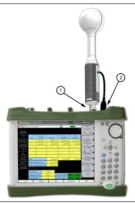
Figure 8-1. Connecting the Anritsu Isotropic Antenna
